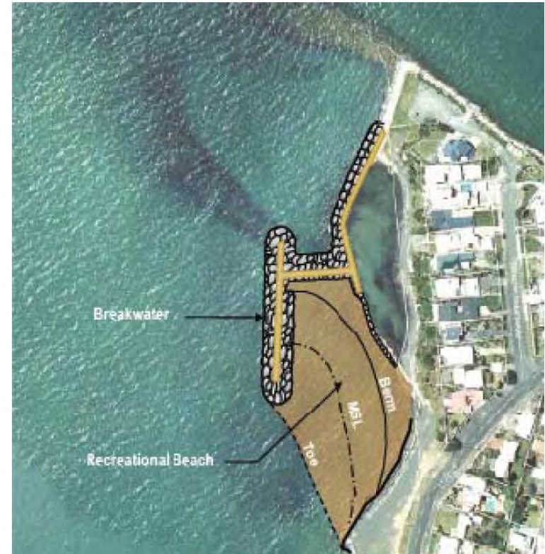
Figure 4.1 H-Shaped Breakwater Layout
